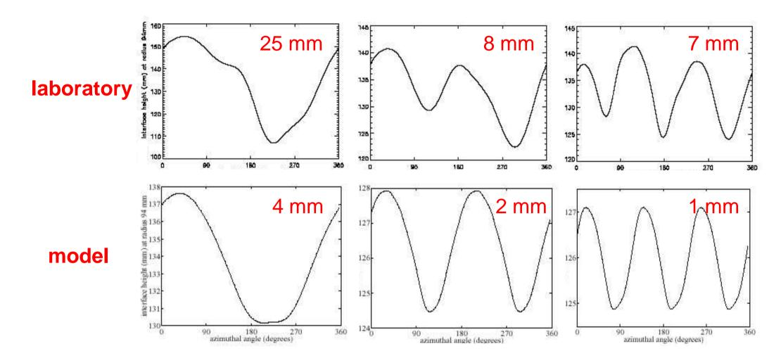
Although the model correctly captures the decreasing amplitude with increasing wavenumber, the model waves are a few times weaker than the laboratory waves and are more monochromatic.
