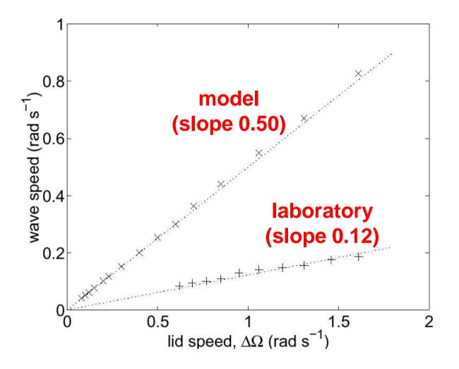
The wave speed is proportional to the lid speed in both the laboratory and the model, but the model overestimates the wave speeds by a factor of around 4.
