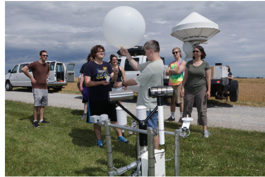
Fig. 2. The SPOTTR 2017 instrument training session. Instructor D. Dawson, holding the balloon, instructs student J. Gable on proper sonde release technique. A PIPS can be seen in the foreground, and the UMass X-Pol radar truck is parked behind the group. From left to right, participants are P. Saunders, S. Simmons (hidden), J. Gable, A. LaFleur, instructor D. Dawson, K. Popp, and instructor R. Tanamachi. Photo courtesy of T. Uhlman.
