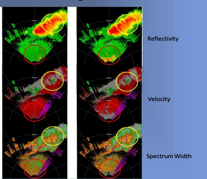
The RVW image shows how the moments (R,V,&W) with near-zero velocities from a meso-cyclone (yellow circles) are not harmed by the CLEAN-AP filter; while, ground clutter near the radar is mitigated quite nicely.
