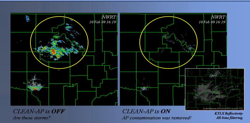
The AP image shows a comparison of the KTLX radar with the NWRT PAR. The environment exercised the capability provided by the CLEAN-AP filer to automatically mitigate (detection and removal) ground clutter in both AP (yellow circle) and NP (near radar) conditions. The KTLX radar ran all bins clutter filtering to remove the AP ground clutter.
