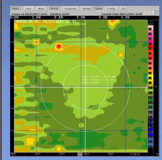
External targets can be used to improve calibration and monitor stability. Shown here are H and V solar power scans. (Courtesy Mike Dixon, NCAR)
