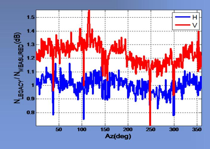
Legacy to radial measured noise ratio in the horizontal (H), and the vertical (V) channel.
