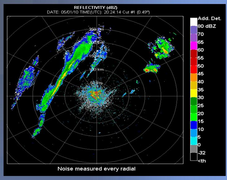
Reflectivity field obtained using the radial based noise measurement with additional detections highlighted in white.
