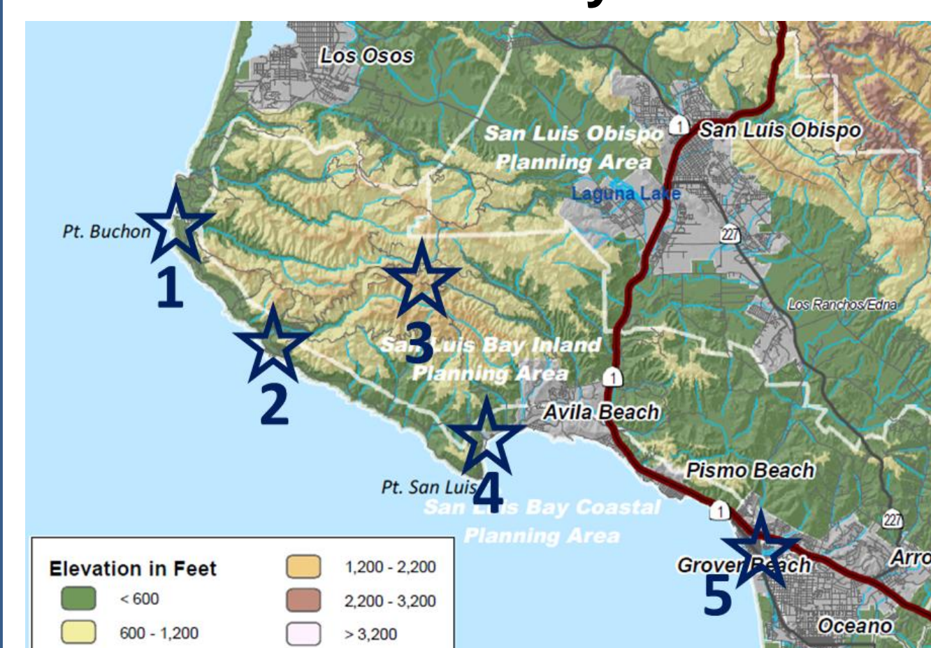
Fig. 6 Terrain that produced the Grover Beach eddy, with the locations of relevant monitoring stations superimposed and numbered as follows, PG&E 1-3: 1) Pt. Buchon 2) Diablo Canyon Nuclear Power Plant meteorological tower 3) Davis Peak; 4) Cal Poly pier; 5) SLOAPCD Grover Beach site. Ridges extend to between 450 to 550 m (1500-1800 feet) MSL. Base map courtesy of San Luis Obispo County Planning Department, Geographic Technology and Design Section.
