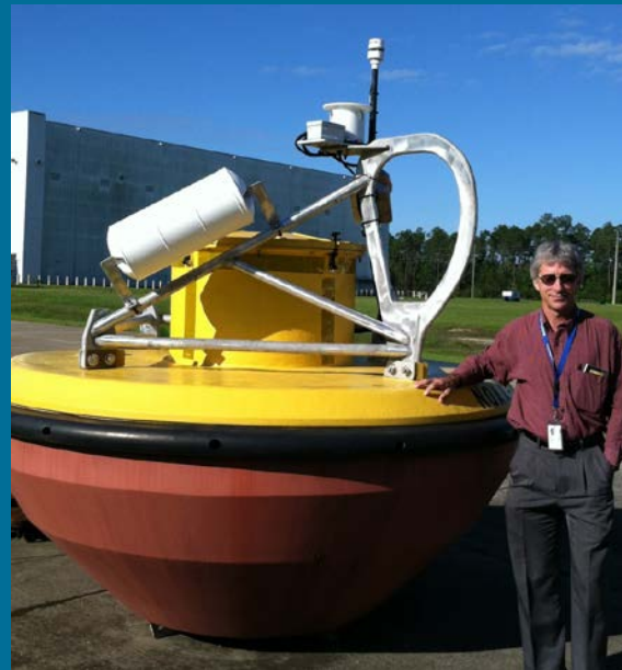
Generation 1 BuoyCAM and MET on DART Buoy
