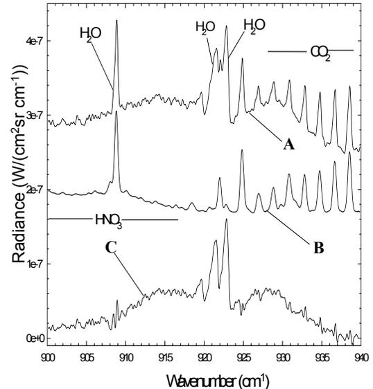
**Figure 2.** The extraction of the thermal emission band of CFC-12 from the measured atmospheric emission spectrum (curve A). Curve B represents the simulated background thermal emission in the
