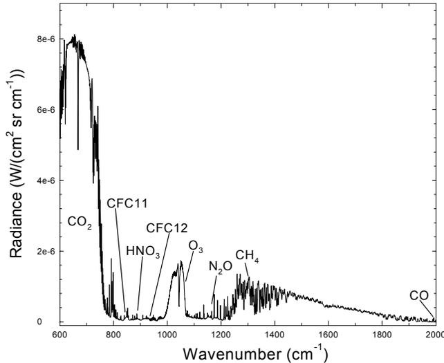
**Figure 1.** A spectrum of the greenhouse radiation at the surface measured for February, 1996, showing the contributions of several greenhouse gases.
