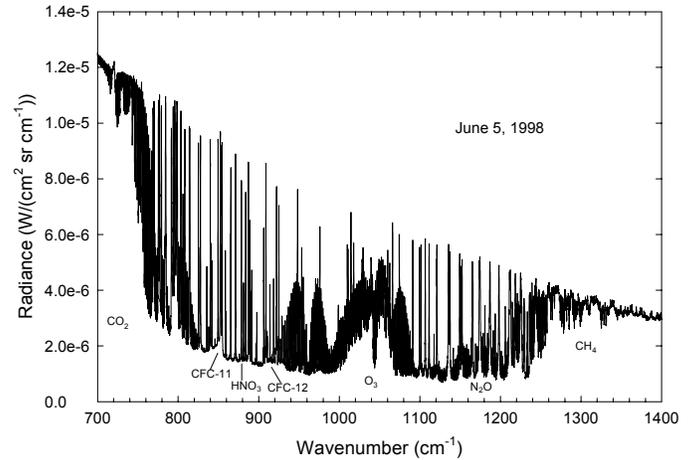
**Figure 3.** A spectrum of greenhouse radiation forcing measured in summer showing enhanced water lines.
