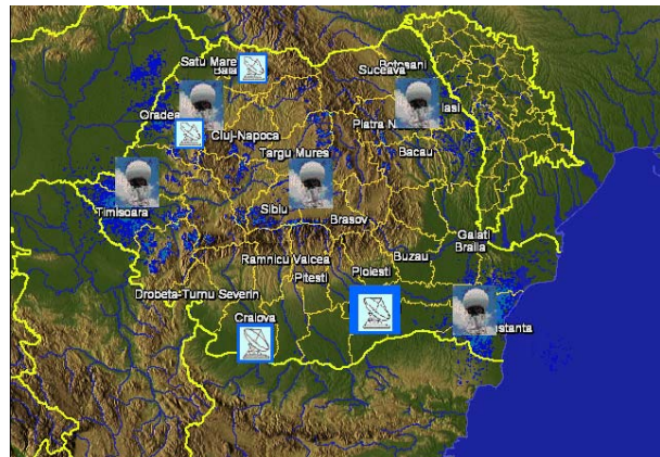
Fig. 1: The Romanian National Radar Network integrates: 5 WSR-98D S-band radars (a clone version of WSR-88D radar used in US NWS network) and 3 C-band radars (2 from EEC – DWSR-2500C type and 1 from Gematronik – METEOR 500C type).
