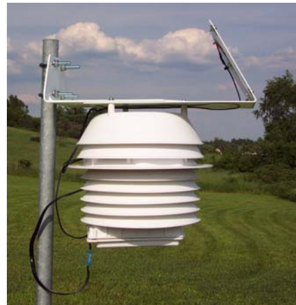
FIG. 2. Vantage Pro Temperature/Humidity Station retrofitted with a Daytime Fan-Aspirated Radiation Shield Kit
