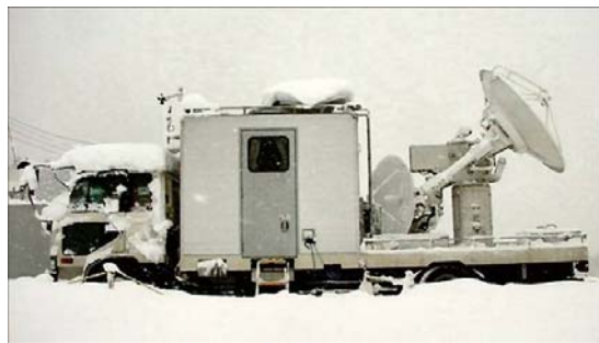
FIG. 2. A photograph of the NIED MP-X radar.
