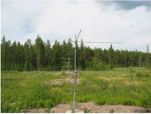
Figure 3: A photograph of the antenna field of the SKiYMET meteor radar located at Esrangle. The radar system comprises five receive antennas, as well as a transmit antenna, covering an area of approximately 2000 m 2 .
