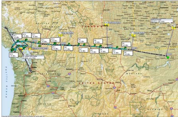
Figure 4: Flight path from Glasgow Montana to Mt Sicker, BC radar site. Black dots indicate flight path, blue dots are radar detections above the FCC regulatory -62dBm threshold, green flags are radar detections above a -50dBm limit.
