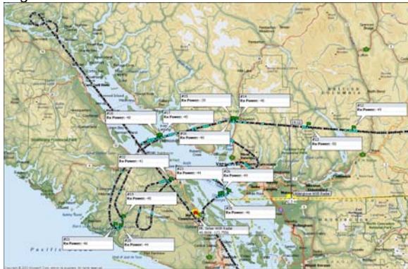
Figure 5: Details of flight path around Mt. Sicker radar site with DFS power readings annotated. Black dots indicate flight path, blue dots are radar detections above the FCC regulatory -62dBm threshold, green flags are radar detections above a -50dBm limit.
