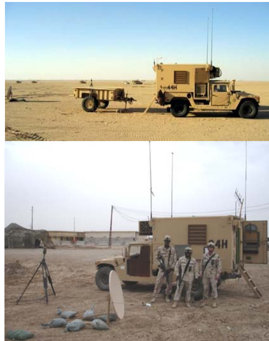
Figure 1. The MMS-Profiler system, housed in a Humvee, on the desert battlefields of Iraq with large guns in the background (top), and with its crew, armed and wearing desert camouflage (bottom). The T-VSAT dish in the foreground of the lower photo provides global model data and WMO regional observations via military satellite communications, and the TACMET weather sensor on the tripod measures surface wind speed and direction, temperature and relative humidity, to be assimilated into the system.
