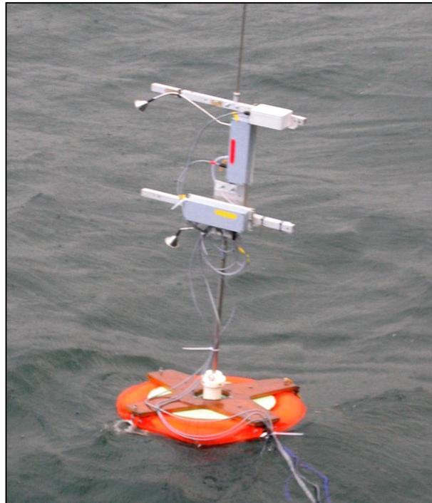
**Figure 4.** The Leeds aerosol buoy. CLASP aerosol probes are located in the grey enclosures with inlets at approximately 0.5 and 1 m; the motion pack .
