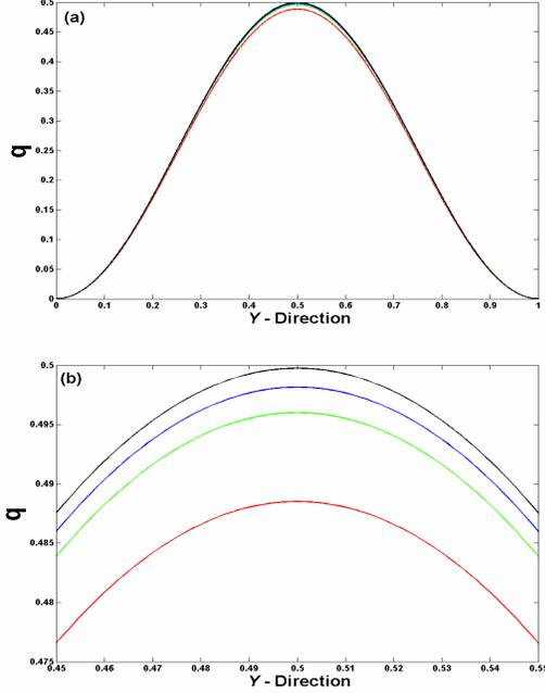
**FIG. 5** Variation of  $q$  in  $y$  direction for various  $Ri$ 's: a) over full domain; b) in center of domain for  $Ri$ : 10: red; 40: green; 100: blue; 1000: black.
