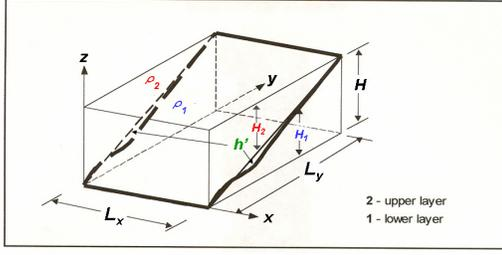
**FIG. 1** Two layer shallow water model schematic. Thin solid and dashed lines represent  $\bar{h}$  and  $\rho_1 > \rho_2$
