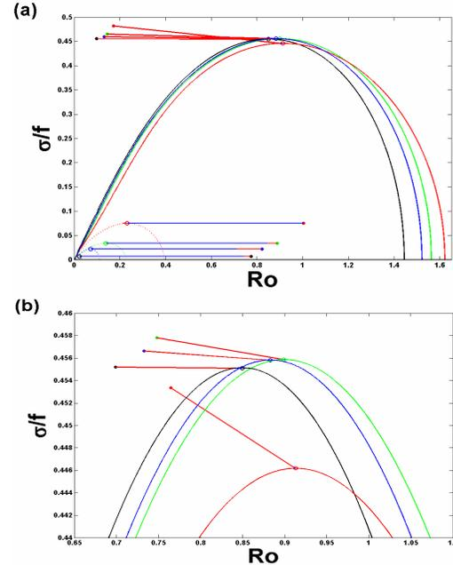
**FIG. 9** Growth rates normalized by  $f$  vs  $Ro$  for the dry mode ( $q_c = 0$ ; dotted) and warm core as most unstable mode (solid) for  $Ri$  10 (red ( $q_c$  0.4885);  $Ri$  40 ( $q_c$  0.496) green;  $Ri$  100 ( $q_c$  0.49815) blue;  $Ri$  1000 (black ( $q_c$  0.49976)). Energy vectors as in Fig. 6. (b) Close-up of warm core as most unstable mode; notation same as in (a).
