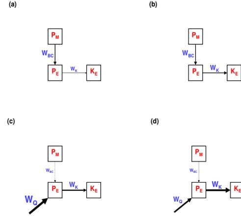
**FIG. 4** Energetics for the cases: (a)  $q = 0$ ;  $Ro \sim O(10^{-1})$ ; (b)  $q = 0$ ;  $Ro \geq O(10^{-1})$ ; (c)  $q > 0.5$ ;  $Ro \sim O(\infty)$ ; (d)  $0.45 < q < 0.5$ ;  $Ro \sim O(1)$ . Font size and arrow shaft thickness for energy conversions are proportional to their relative magnitudes. Dashed  $W_{BC}$  arrow shaft in (c) indicates  $W_{BC}$  is not required in this case.
