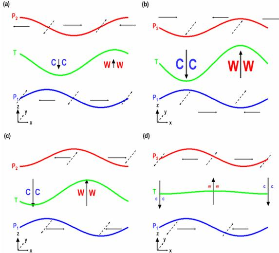
**FIG. 8** Schematic of the four phase lags and associated circulations found for the (a)  $Ro \mathcal{O}(10^{-1})$ ; (b)  $Ro \mathcal{O}(1)$ ; (c)  $Ro \mathcal{O}(>1)$ ; (d)  $Ro \mathcal{O}(>>1)$  cases. Vertical arrow lengths are proportional to strength of vertical velocities. Font size for C's (cold) and W's (warm) proportional to amplitude of interface (thickness) perturbation. Solid arrows perturbation zonal velocity; dashed arrows perturbation meridional velocity.
