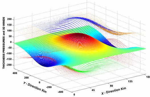
**FIG. 11** Ri 1000 warm core case. Three dimensional perturbation winds projected on upper and lower layer perturbation pressure fields, respectively. Lower layer winds with positive (negative) vertical velocities: green (red). Upper layer winds with positive (negative) vertical velocities: blue (brown). Perturbation thickness field is colored mesh surface ranging from greatest red values to least blue values. Y - direction distances as in Fig. 10.
