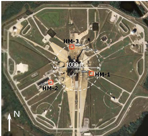
Figure 1. Hail monitor stations at Pad 39A.
