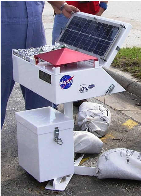
Figure 3. Site 3 hail monitor unit at Pad 39A.
