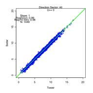
Figure 3 Scatter plot of hourly-averaged sodar 50 m wind speeds against tower 50 m wind speeds.
