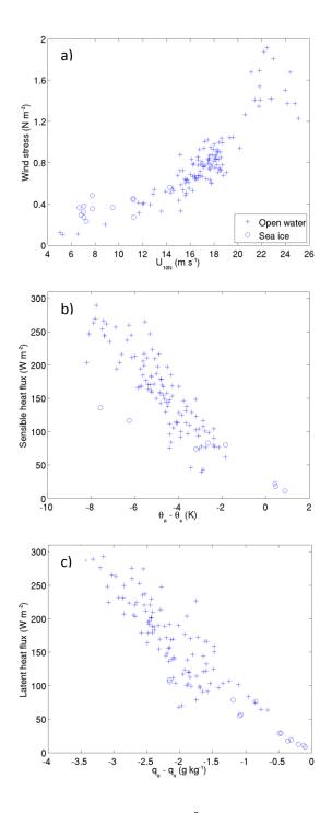
Figure 2: (a) Wind stress  $(Nm^{-2})$  as a function of  $U_{10N}$  (ms<sup>-1</sup>), (b) sensible heat flux (Wm<sup>-2</sup>) as a function of air-sea potential temperature difference (K) and (c) latent heat flux as a function of air-sea humidity difference (gkg<sup>-1</sup>). Flux runs over open water are represented by crosses and those affected by sea ice by circles.
