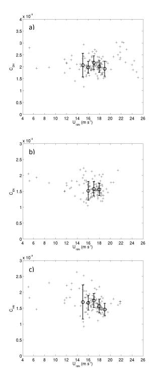
**Figure 3:** 10-m neutral exchange coefficients over open water for (a) momentum, (b) sensible heat and (c) latent heat as functions of the 10-m neutral wind speed (ms<sup>-1</sup>). The 1-ms<sup>-1</sup> bin-mean values are shown for circles and the error bars show one standard deviation. Only bins with at least 10 data points are shown.
