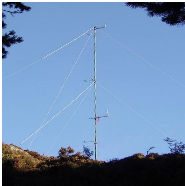
Figure 5. Photo of vertical profile tower at site T1, showing the top two sonic anemometer booms (right) and the top three mean booms (left).
