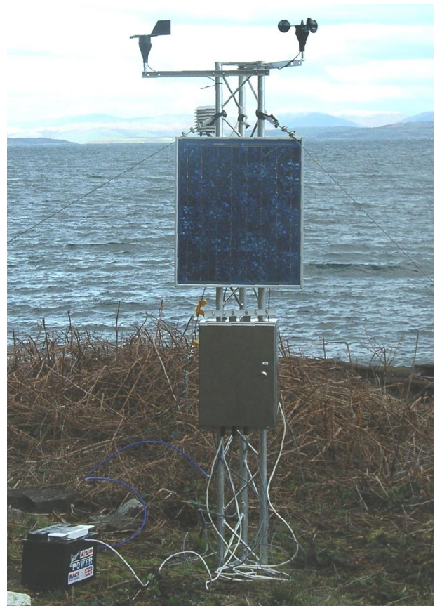
Figure 6. Photo of an AWS at site ARJ showing (from top to bottom) wind vane (left), cup anemometer (right), temperature sensor aspirator, solar panel, logger box, blue lead to pressure sensor and 12v battery.
