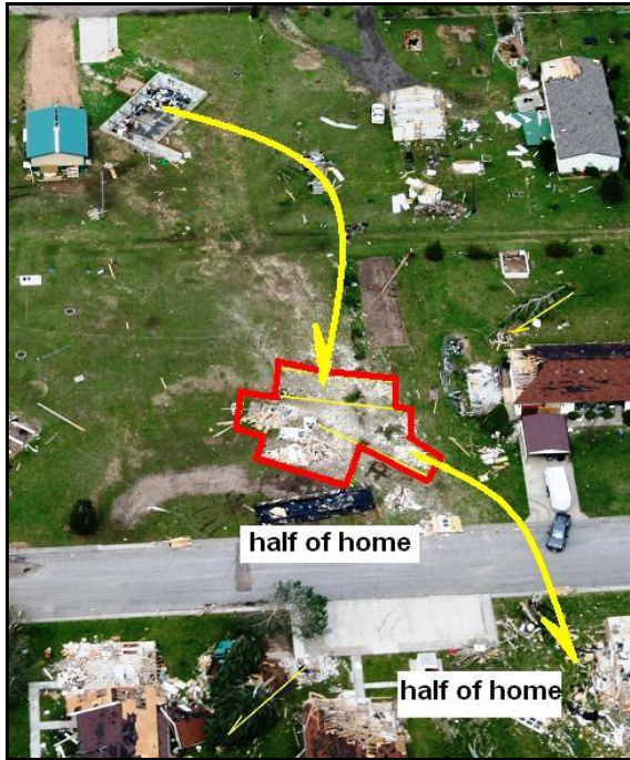
Figure 7. Lofting of unanchored, double wide manufactured home in area where residences experienced only EF-0 to EF-2 damage.
