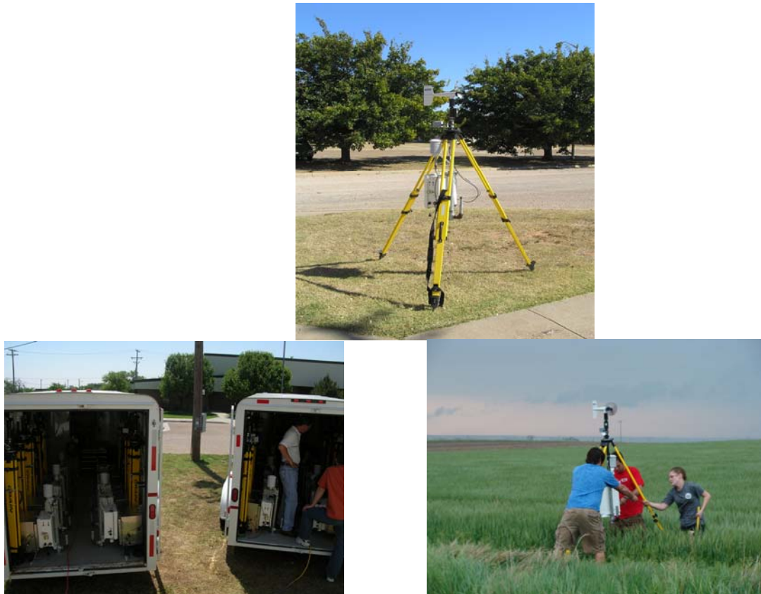
FIGURE 1 – Photographs of a StickNet station (top), transport trailers (lower left) and deployment (lower right) during the MOBILE field project.
