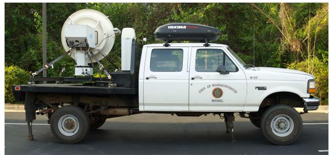
Figure 1: UMass W-band mobile radar.
