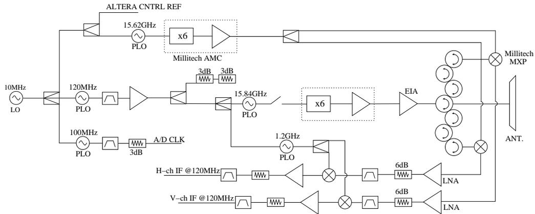
Figure 3: UMass W-band radar system diagram.
