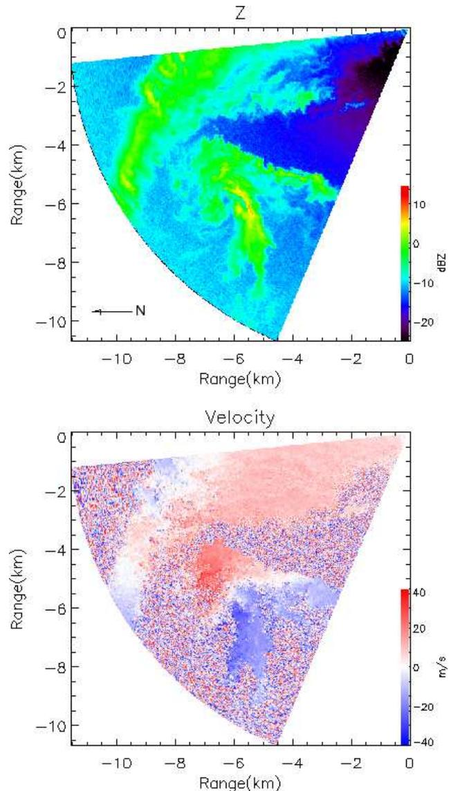
Figure 4: A PPI scan from UMass W-band radar at 2157 UTC, May 23, 2008. The elevation angle is  $0.446^\circ$ . Upper: reflectivity, lower: velocity
