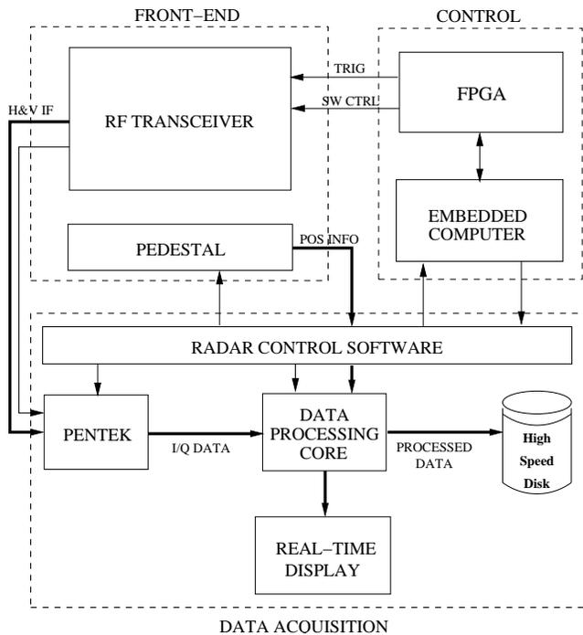
Figure 2: UMass W-band radar subsystems and signal flow.
