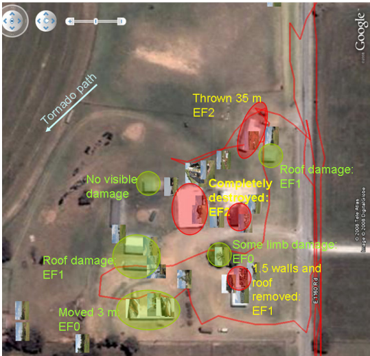
Figure 7. A ground-based survey of structures at a farmstead near Minco, OK from a tornado on 2007 August 19. The red trace represents the path of the surveyor took to investigate the structures. Pictures were geotagged and placed in a KML file to be displayed in Google Earth.
