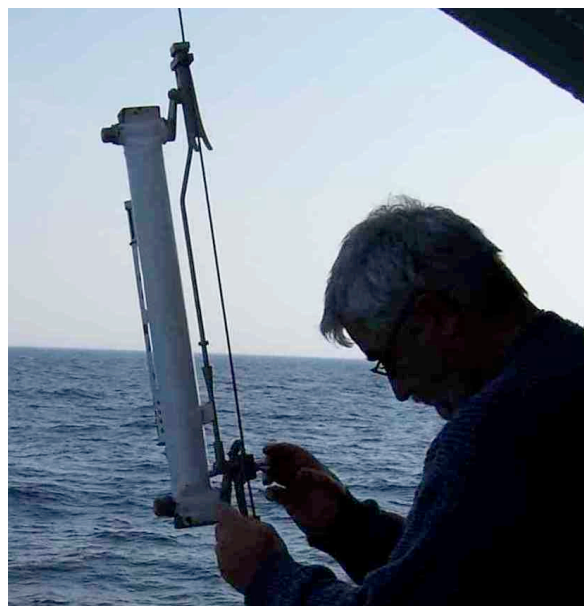
Figure 2. One of the Polarfront crew preparing the Nansen bottle.
