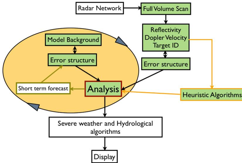
Fig. 2- Block diagram of the Mesoscale Analysis System. The green panels show implemented elements (some at a very elementary stage), white panels show work yet to be initiated. The cycle of assimilation is in orange.
