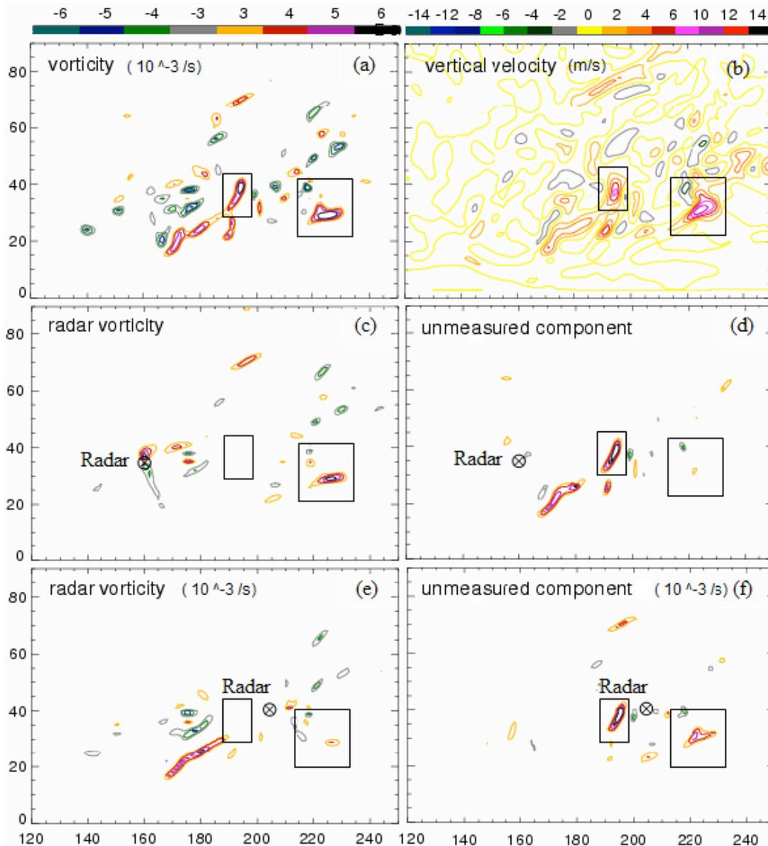
Fig. 1 - The upper two panels show the fields of vorticity and vertical air velocity computed from numerical simulations of a tornadic storm. Model (MC2) resolution was 1km. The other panels show the vorticity of the radar radial wind component (left) and the vorticity of the tangential wind component (right) at the indicated radar positions.
