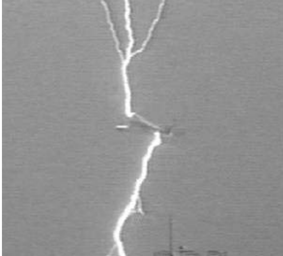
Figure 2: Aircraft hit by lightning. Photograph found on the internet. Reprinted and discussed by Uman and Rakov (2003).
