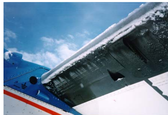
Figure 4: wind shield and wing icing after a flight of the DLR Dornier 228 aircraft in severe icing conditions.
