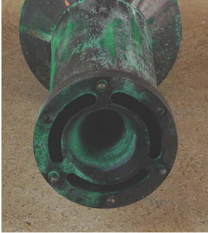
Figure 15: Photograph of the lower end of a Dines anemometer float, showing the choke. The pressure tube enters up the hole in the middle, almost filling it.
