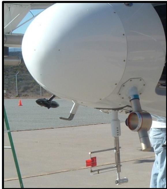
**Fig.2.** UFT-M thermometer (red vane) mounted below the nose of CIRPASS Twin Otter research aircraft.
