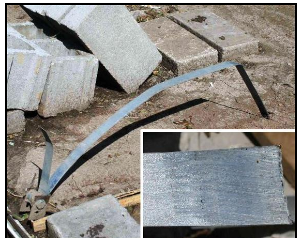
Figure 15. Broken strap on an auger anchor. The inset image shows scrape marks on the strap indicating movement of the steel undercarriage occurred prior to strap failure.
