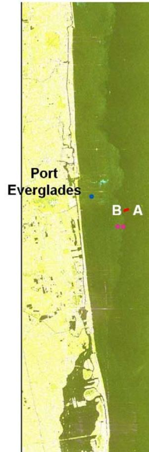
**Figure 6: TerraSAR-X image acquired on June 10th, 2010 (11:17 GMT). SAR data was acquired in dual polarimetric mode (HH-VV combination), with HH for red color, VV for green color, HH-VV for blue color. Location of CTD casts is indicated by purple dots, AWAC by blue dot, and track of boat by red line between 'A' and 'B'.**
