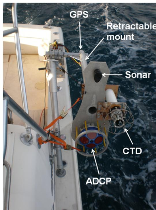
Figure 1: Retractable mount for sonar, GPS, ADCP, and CTD instruments.
