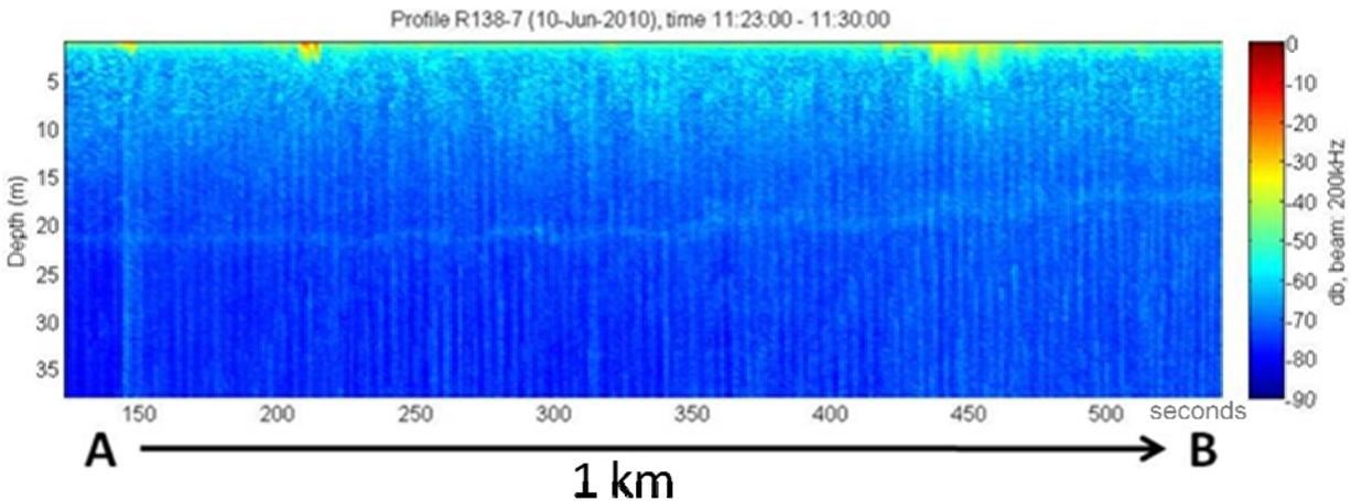
**Figure 4: Sonar plot taken from 11:23 to 11:30 GMT on June 10th, 2010. This sonar transect was collected by travelling towards shore a distance of 1.6km from point 'A' to 'B' as shown on the plot and the SAR image. Plot shows a thermocline located at approximately 20 meters depth.**
