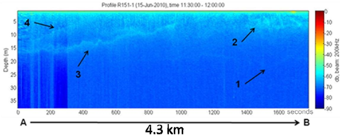
Figure 13: Horizontal sonar cross-section showing a front surfacing. This sonar transect was collected by travelling towards shore a distance of 7.1 km from point 'A' to 'B' as shown on the plot and the SAR image. Features indicated on the plot are as follows: 1-thermocline, 2-microstructure in the near surface layer, 3-frontal interface, 4-acoustic artifact relating to bottom reflection due to late echoes (see Section 2 for details).
