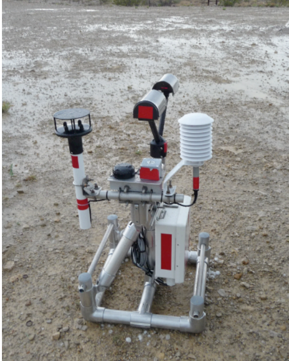
Figure 2. One of the two Parsivel disdrometer probe packages, seen shortly after a deployment.
