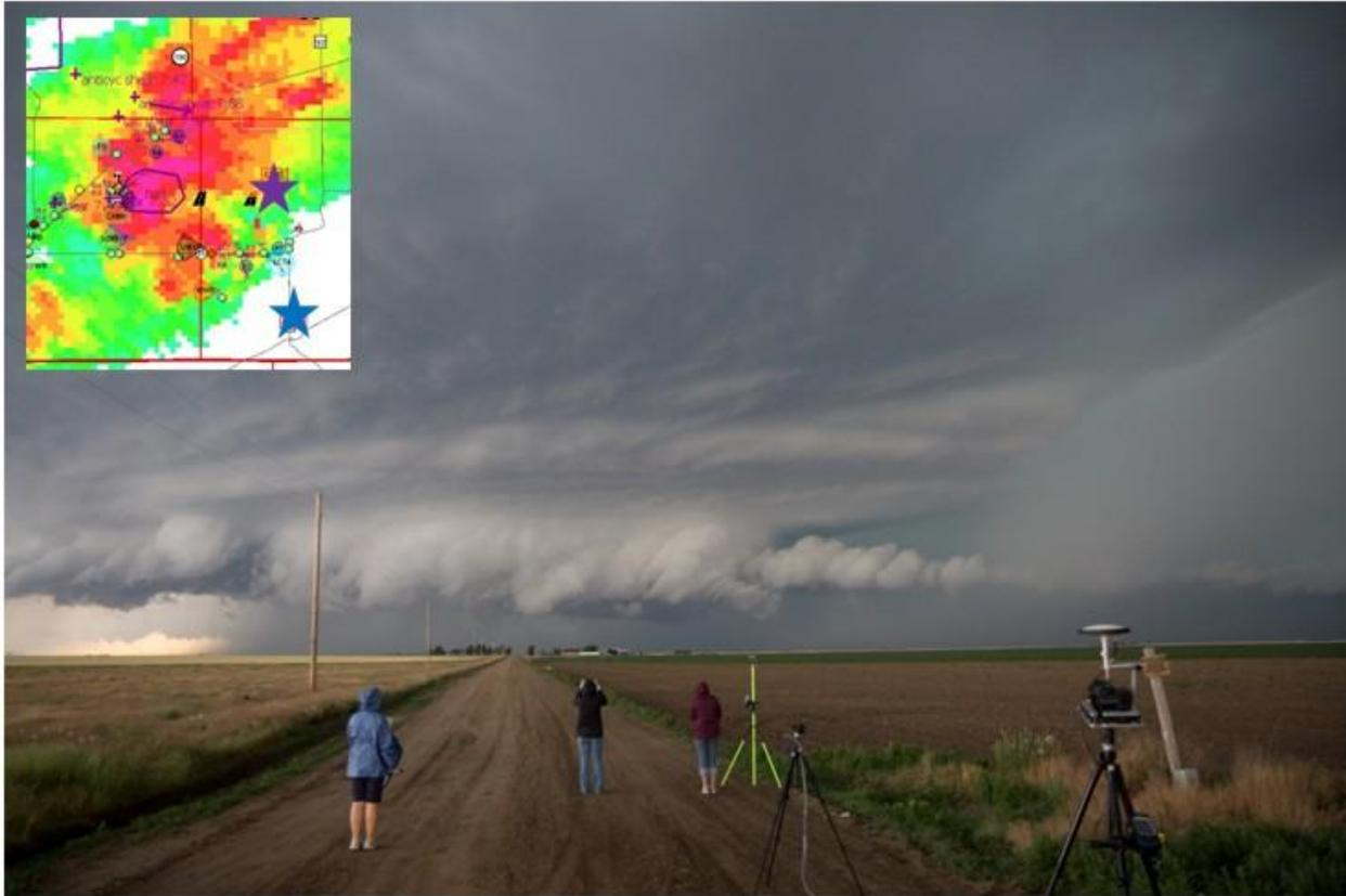
Figure 4. Front side deployment on an HP supercell on Jun 10, 2009 with camera base station (lower right) and rover GPS on yellow bipod (center). Also shown is an intermediate tripod holding a water hose used as a redundant measure of horizon. Radar reflectivity (upper left) with team positions (stars) shows where camera was located (purple star).
