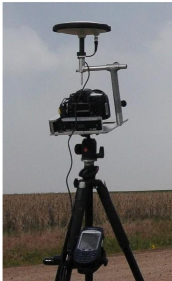
Figure 1. The photogrammetry camera base station including: 1) Promark3 GPS (bottom), GPS antenna (top), Nikon D300 camera fixed to a custom-built tripod mount with digital protractors on the rear and left side of the mount to measure pitch and roll.
