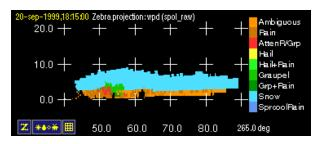
**Figure 4**. Precipitation particle types identified by the Zeng et al. (2001) algorithm based on a vertical cross section (RHI) scan made by the multiple-polarization S-Pol radar on 20 September 1999 at 18:15 UTC in the direction 265 azimuth.
