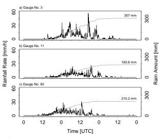
**Figure 1.** Rainfall rate and accumulation traces recorded during the 19-21 September 1999 heavy rainfall event by three gauges (placed within 2 km) near the outlet of the Anza river valley (see Fig. 2).
