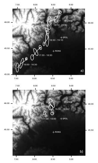
**Figure 2**. Tracking analyses based on Mt. Lema radar data for storms occurring on 20 September 1999. Shown are examples of two types of tracks: **a)** northeastward, along-barrier propagating cells from 16:00-20:30 UTC and **b)** quasi-stationary cells from 15:30-19:30 UTC. The 3 triangles ( $\Delta$ ) indicate the location of the special gauges (Fig. 1).
