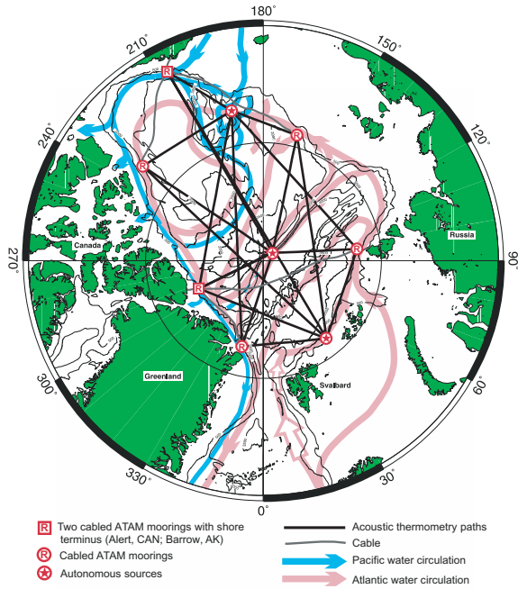
Fig. 8. A future notional monitoring grid in the Arctic Ocean with instruments cabled to shore at Alert, Canada, and Barrow, Alaska. ATAM stands for Acoustic Thermometry and Autonomous Monitoring.
