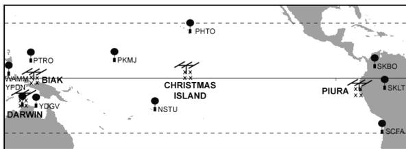
**Fig 1.** The Trans-Pacific Profiler Network. Antenna symbols mark the locations of wind profiling radars at Darwin, Biak, Christmas Island, and Piura. Balloon symbols mark the nearest rawinsonde launch sites. The crosses mark the closest four reanalysis grid points around the profiler site. A solid line marks the equator, while dashed lines mark the Tropic of Capricorn and the Tropic of Cancer.
