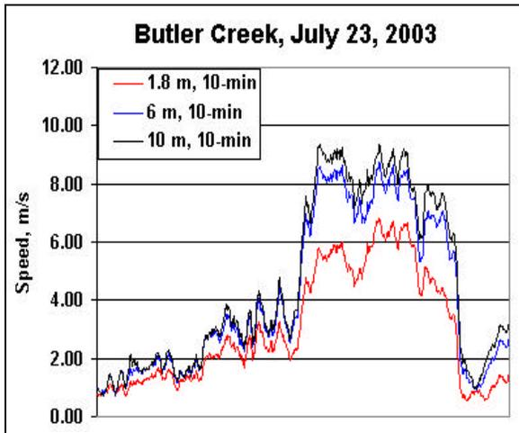
Figure 4. 10-minute wind speeds at 3 heights, every minute from 0900 to 2300 on 07/023 at Butler Creek.
