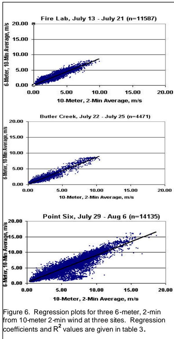
Only the Point Six data set has any scatter of significance—an under prediction for a subset of 10-m, 2-minute winds speeds from about 5 to 8 m/s. An initial look at this subset indicates this is probably a time-lag effect between the 2 and 10 minute averages at the onset of gustiness and increasing winds. A similar, but less apparent lag effect is above the trend line at the higher wind speeds when winds start subsiding.
