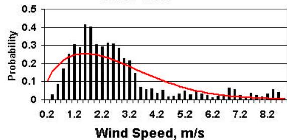
Figure 2. Histogram of Butler Creek wind speed with fitted Weibull distribution function ( $\alpha=1.59$ ,  $\beta=2.97$ ,  $n=4471$ )
