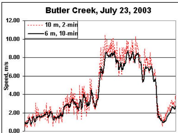
Figure 5. 10-meter, 2-min. and 6-meter 10-min. average wind speed from 0900 to 2300 at Butler Creek.
