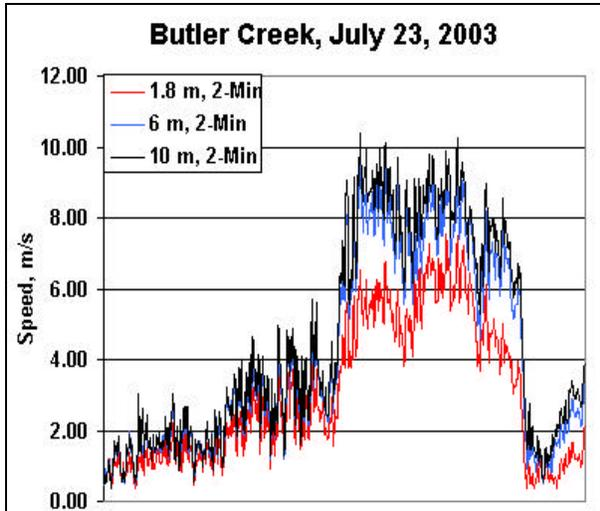
Figure 3. 2-minute wind speeds at 3 heights, every minute from 0900 to 2300 on 07/023 at Butler Creek.
