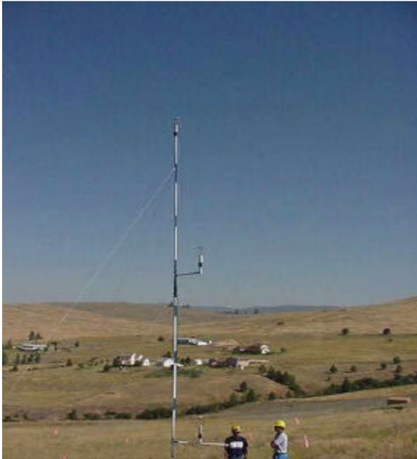
**Figure 1.** Portable anemometer tower at Butler Creek. Instruments are at 1.8, 6, and 10 meters above ground.
