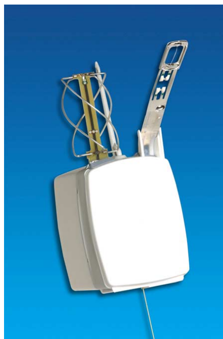
Figure 1. The new Vaisala RS92 GPS radiosonde with its modular mechanics.
