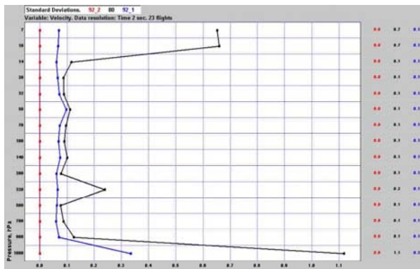
Figure 4. Wind speed (velocity) standard deviation of differences of two RS92-SGP radiosondes and one RS80-15G radiosonde.
