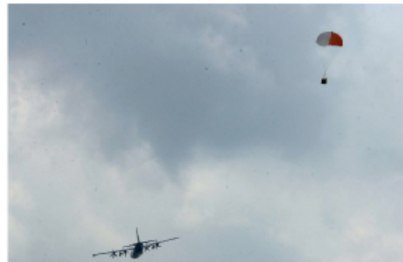
Figure 1. Box containing two Minimet drifting buoys is deployed from an AFRC 53 rd Weather Squadron WC-130J.
