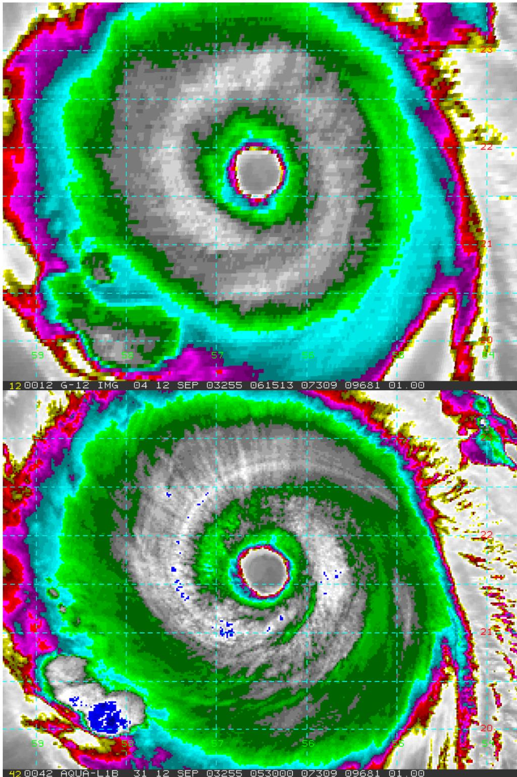
Figure 4: Images of Hurricane Isabel mapped into a Mercator projection. Top image is a GOES-12 infrared image at 4 km resolution. Bottom image is a MODIS infrared image at 2 km resolution, the spatial resolution expected of the GOES-R ABI.
