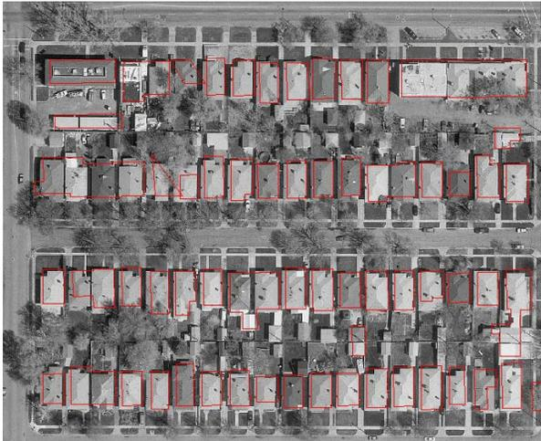
**Figure 1.** Sample residential area in Salt Lake City. Red outlines represent a vector dataset derived through an automated analysis of a full-feature DEM.
