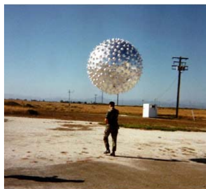
Fig. 1. Jimsphere balloon used for high resolution wind measurements.
