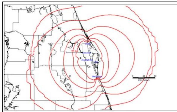
Figure 3. Location accuracy (km) (50% confidence) under the best five-sensor configuration (with Duda/Deseret Ranch sensor not available). Isopleth values are for 0.3, 0.5, 1.0, 2.0, 4.0, and 8.0 km.
