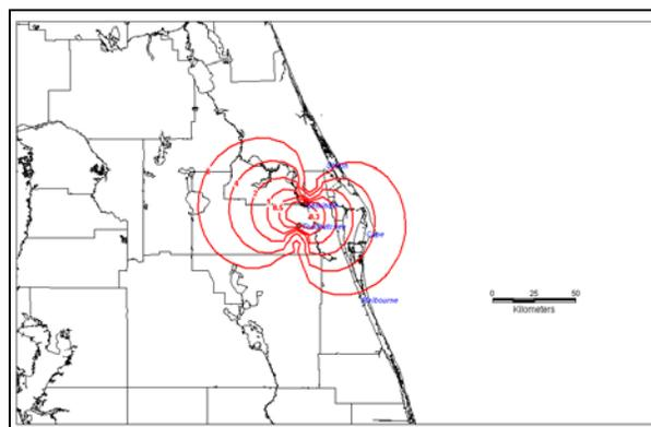
Figure 4. Location accuracy (km) (50% confidence) under the worst two-sensor configuration (with Duda/Deseret Ranch sensor not available). Isopleth values are for 0.3, 0.5, 1.0, 2.0, 4.0, and 8.0 km.
