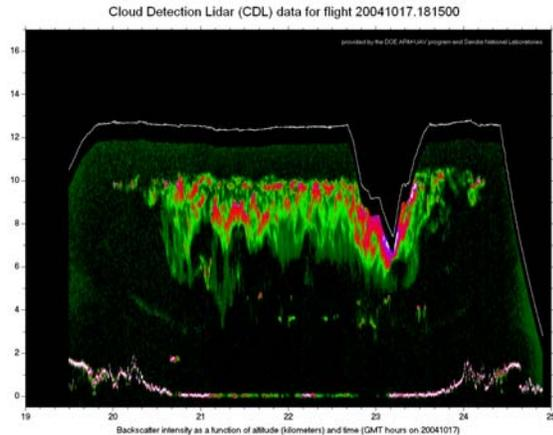
**Figure 13:** Cloud detection lidar image from the Proteus lidar. Proteus flight altitude in white.
