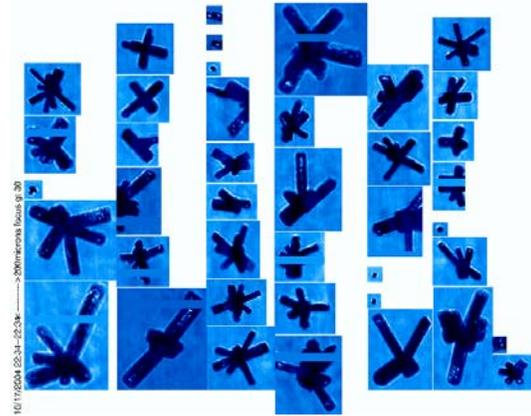
**Figure 15:** Hydrometeor images from the Cloud Particle Imager from October 17.
