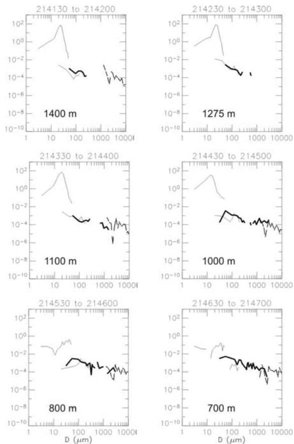
**Figure 9:** Particle size distributions as a function of height as measured by the FSSP, 1DC, 2DC and HVPS (in order of increasing size). Note the presence of bigger particles throughout the depth of the cloud. All data are preliminary and may change with future quality control.
