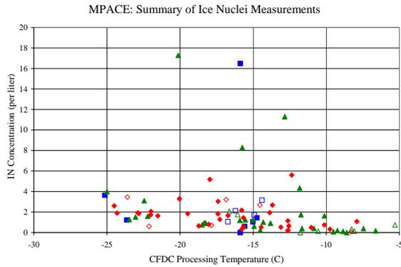
**Figure 11:** Ice nuclei concentration as a function of CFDC processing temperature. Data are presented for measurements taken in clear air and above cloud top (diamonds), in cloud (triangles), and below cloud base (squares). Data are shown for measurements taken above (filled) and below (open) water saturation. All data are preliminary and may change with future quality control.
