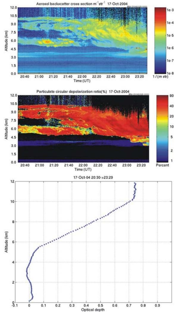
**Figure 12:** Calibrated aerosol backscatter, particulate depolarization ratio, and mean optical depth from the University of Wisconsin HRSL
