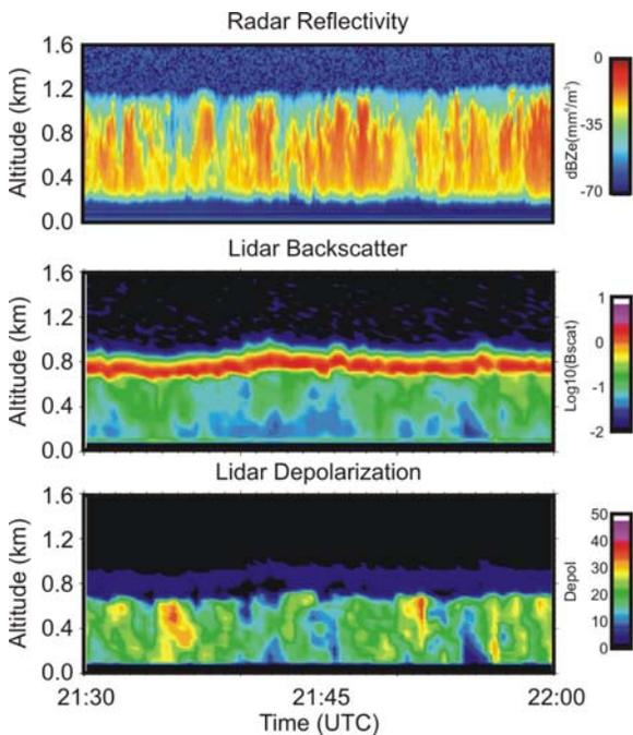
**Figure 6:** PARSL radar reflectivity (top), lidar backscatter (middle) and depolarization (bottom). All data are preliminary and may change with future quality control.
