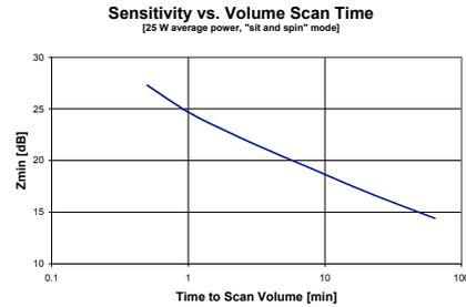
Figure 6. Radar sensitivity (minimum reflectivity causing 1 dB RMS reflectivity error at  $R_{max}$ ) versus volume-scanning update time for the geometry shown in Fig. 5.
