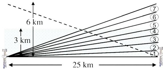
Figure 5. Volume coverage pattern comprised of 7 elevation beam positions spanning 0-12° in 1.7° steps for observing the lower-troposphere below 3 km altitude. The “cone of silence” above each radar is observed by adjacent radars in the network.
