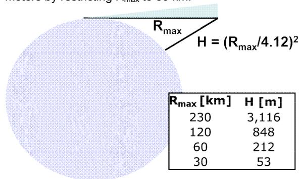
Figure 1. Coverage floor versus radar maximum range.
