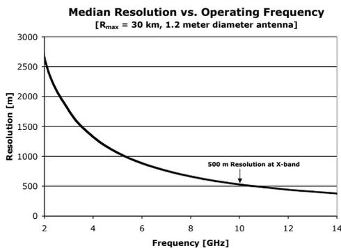
Figure 4. Cross-range (azimuth and elevation) resolution versus frequency for a 1.2 meter antenna. Values shown represent median resolution achieved for radars having  $R_{max}=30$  km. Worse-case resolution is 41% larger than the values shown.
