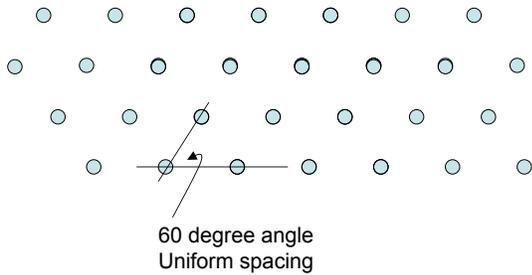
Figure 3. Hexagonal network topology that maximizes dual-Doppler coverage.
