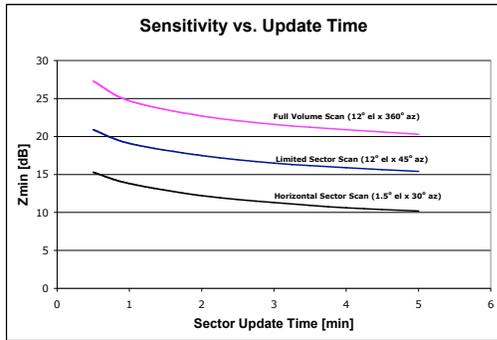
Figure 7. Comparison of three volume coverage patterns revealing the integration-gain benefits accrued by limiting the sectors covered.
