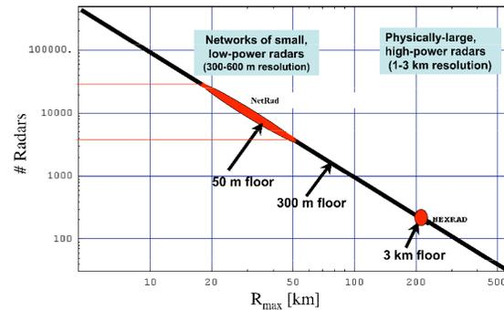
Figure 2. Number of radars needed for nation-wide deployment versus radar spacing.
