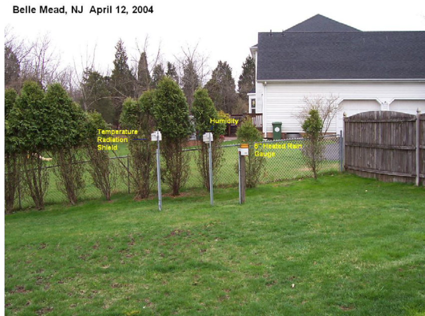
Figure 4. NJ SafetyNet Hillsborough/Belle Mead station. An anemometer is mounted on a nearby chimney.
