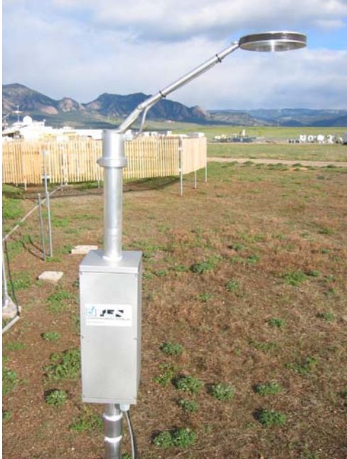
Figure 3 Commercial version of the hotplate snow gauge deployed at the NCAR Marshall Field Site just south of Boulder, CO.
