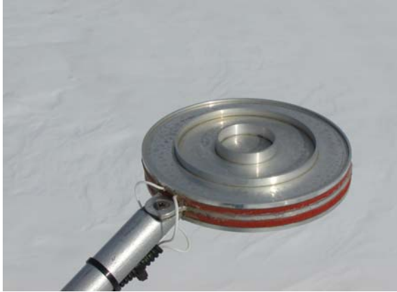
Figure 1 Top view of hotplate. Diameter of plate is 13.0 cm.
