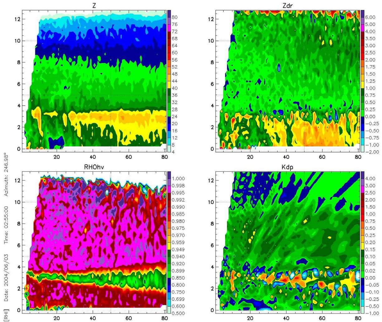
Figure 3: KOUN polarimetric RHI for a 3 June 2004 event which features a prominent melting layer signature and highlights beam broadening.
