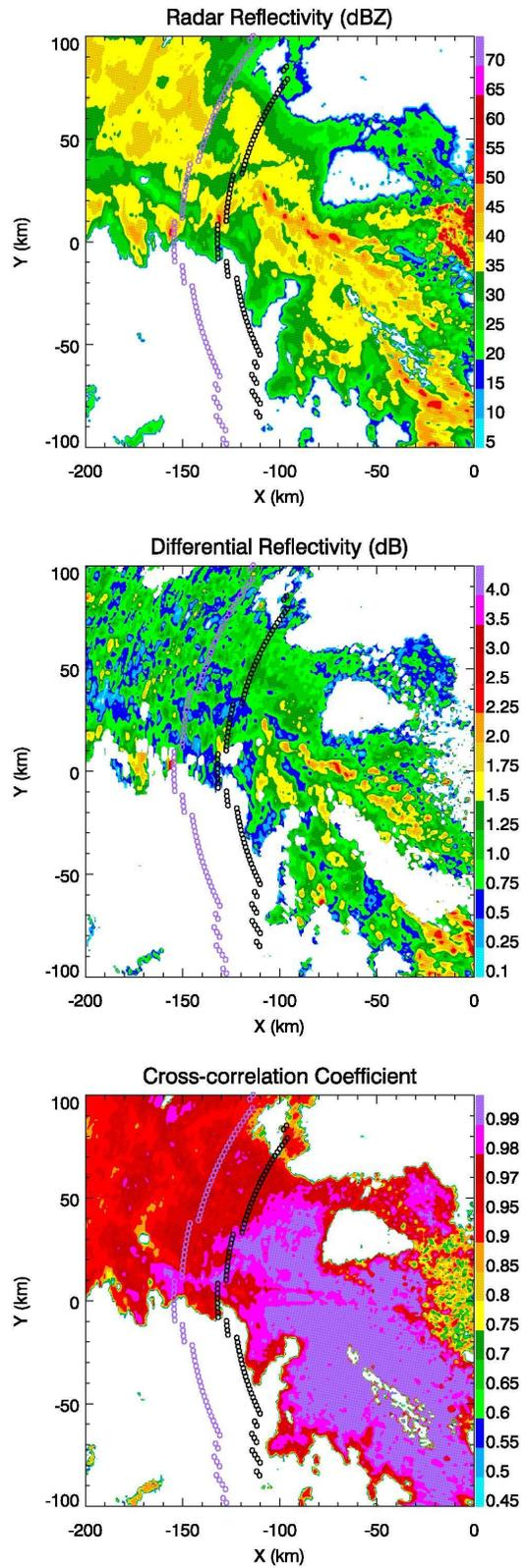
Figure 4: Results of direct(black) and modified(purple) projections of melting layer bottom detection heights to KOUN PPI fields at the 0.5 degree elevation angle.
