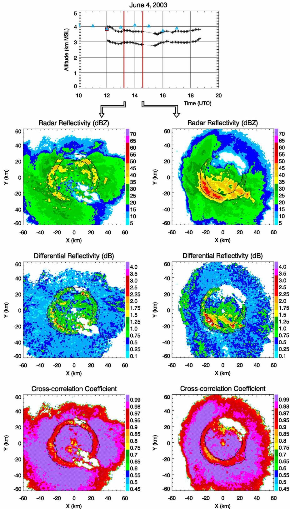
Figure 1: (Top) Mean melting layer top and bottom detections as a function of time for the 4 June 2003 event. Triangles indicate RUC model analysis output freezing level heights for the KOUN location. Red square indicates the local NWS OUN sounding freezing level height. (Bottom) Select KOUN PPI images (times denoted with red lines) with overlaid melting layer detections.
