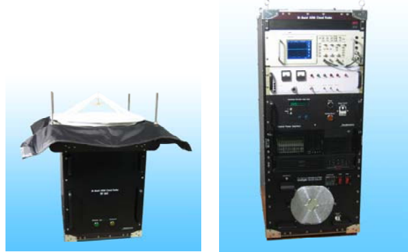
Figure 1. 95 GHz W-band ARM Cloud Radar ceiling mounted upper rack containing RF Unit and antenna (left) and lower rack (right) containing RF unit chiller, data system, UPS, modulator controller and digital scope for transmit sample display.
