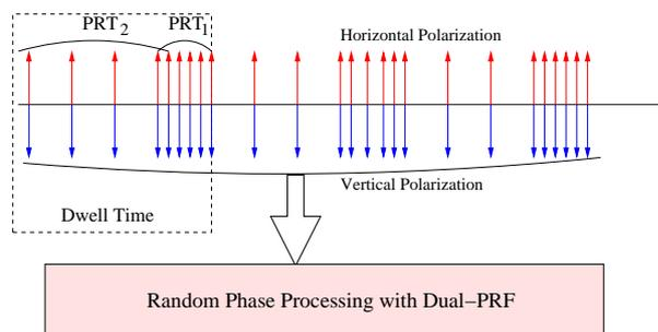
Figure 10: Staggered pulsing with random phase processing
