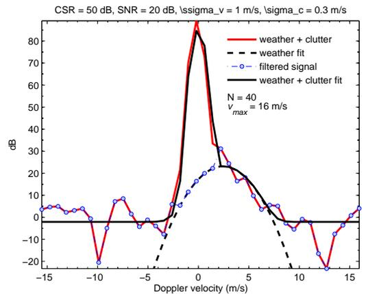
Figure 2: Clutter filtering with bimodal spectral distribution fits
