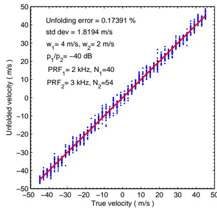
Figure 11: Scatter plot of true vs unfolded velocity with  $PRF_1 = 2$  kHz and random phase processing with  $PRF_2 = 3$  kHz
