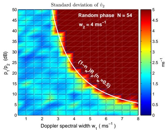
Figure 8: Standard deviation of weak trip velocity after random phase processing with PRF=3 kHz
