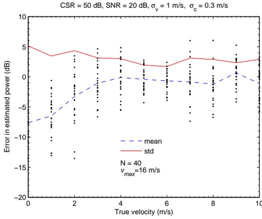
Figure 3: Bias and standard deviation of power after ground clutter filtering
