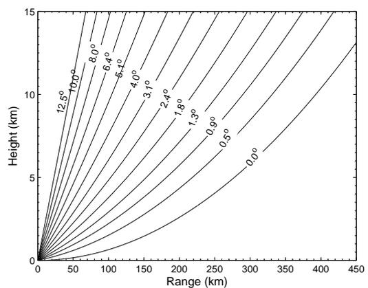
Figure 9: The height of the radar beam center as a function of elevation and range
