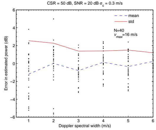
Figure 5: Bias and standard deviation of power after ground clutter filtering as a function of Doppler spectral width
