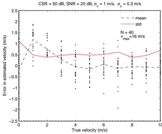
Figure 4: Bias and standard deviation of velocity after ground clutter filtering
