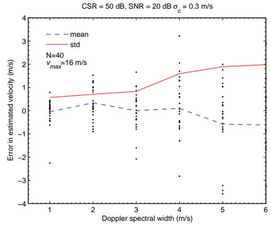
Figure 6: Bias and standard deviation of velocity after ground clutter filtering as a function of Doppler spectral width
