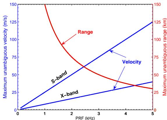
Figure 1: Comparisons of range-velocity limitations for S-band and X-band radars
