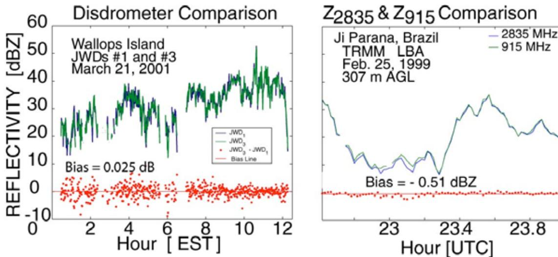
**Figure 4:** The **left panel** shows overlaid time series of the simultaneous observations from two collocated disdrometers. The red dots show the minute-by-minute differences between them. Although the minute-by-minute differences are large (standard deviation =  $\sim 3$  dBZ) the 12 hour means differ by only 0.25 dBZ. The **right panel** shows a similar display for two collocated radar profilers, but at a different time and place. Here the 1 hour means differ by only 0.51 dBZ.
