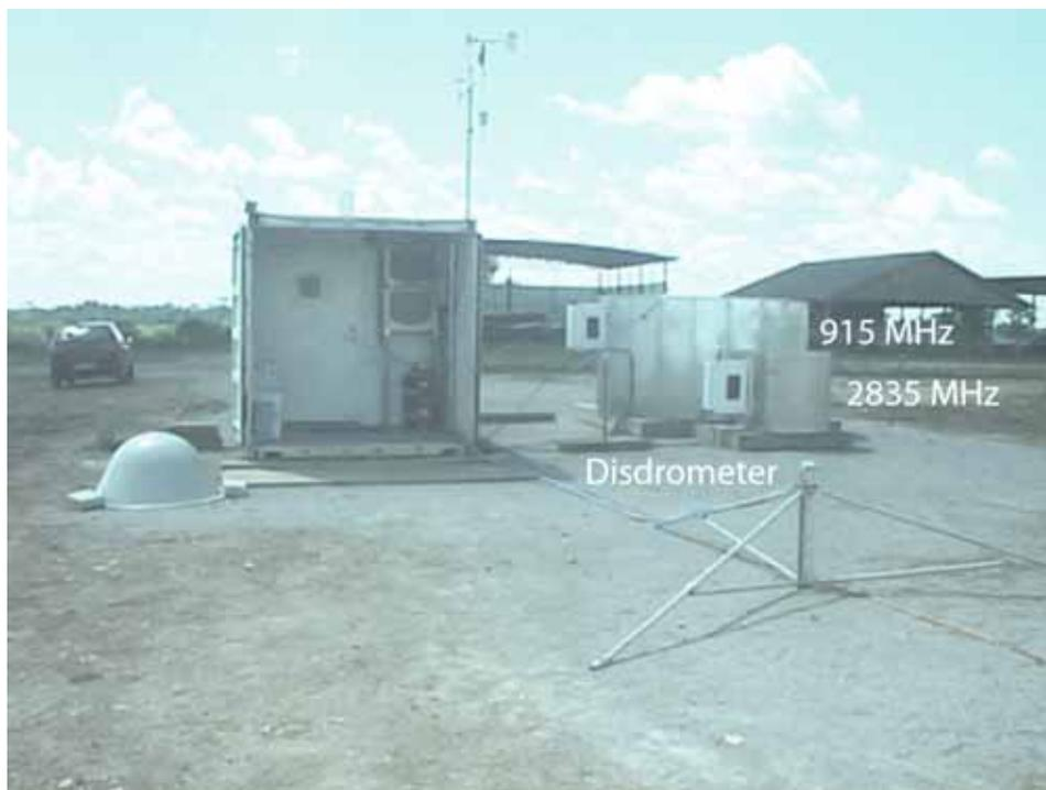
**Figure 2:** From left to right are the radar control container, the 915 MHz profiler antenna shroud and transmitter, the smaller 2835 MHz antenna shroud and transmitter, and the Joss-Waldvogel disdrometer in the right foreground, sitting on a tripod 1 m off the ground.
