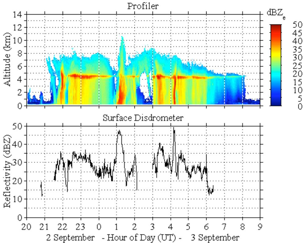
**Figure 3:** Example of the 915 MHz profiler time height display of Z at Legan Island in the Kwajelein Islands. The data are for September 2-3, 1999. A time series of the minute-by-minute Z values observed by a collocated Joss-Waldvogel disdrometer are shown in the bottom panel.
