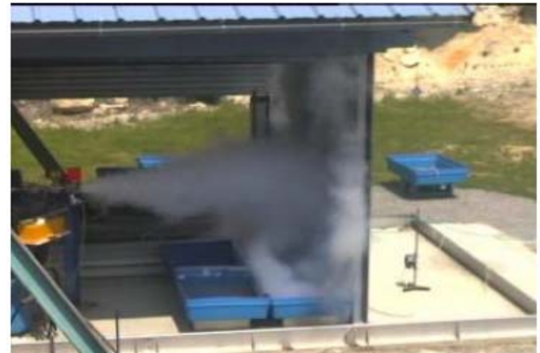
Flashing impinging jet from the INERIS test series report
